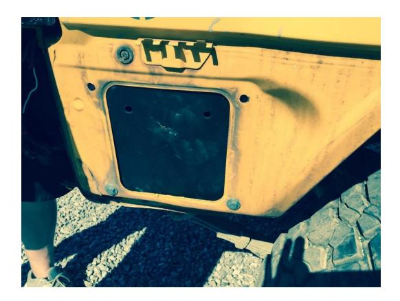
(5) Put 2 more bolts with washers through the upper 2 holes. Have your lovely assistant place and hold a washer and lock nut on the back of these 2 bolts and tighten.
