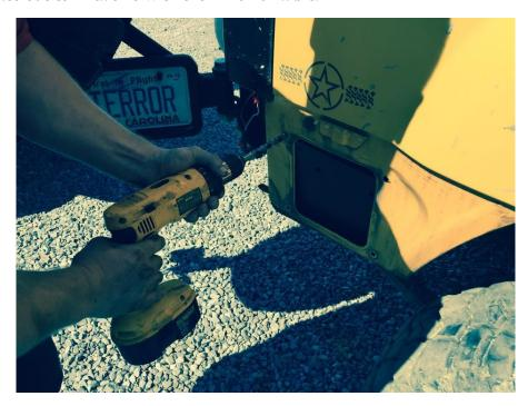
d. Drill the 2 holes out on the pinch seam that held the original corner support bracket using a 7/16" drill bit.
