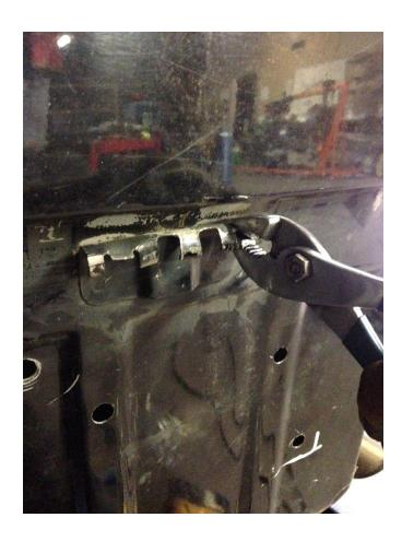
b. Put 2 bolts with washers through the upper mount in the middle of the corner then through the structural inner panel. Have an assistant loosely add a washer and lock nut to the two bolts through the hatch.
