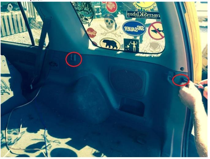
c. Pull out panel while undoing clips along seam between upper and lower trim panels
