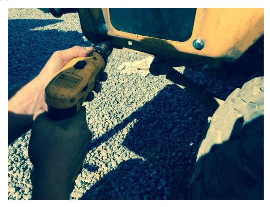
(4) Place structural inner panel into pocket between inner and outer body sheet metal through the access hole in the rear hatch. Make sure the two welded nuts are facing down. Loosely place 2 bolts with washers through the holes drilled in the sheet metal of the truck and thread them into the nuts welded to the structural inner panel.
