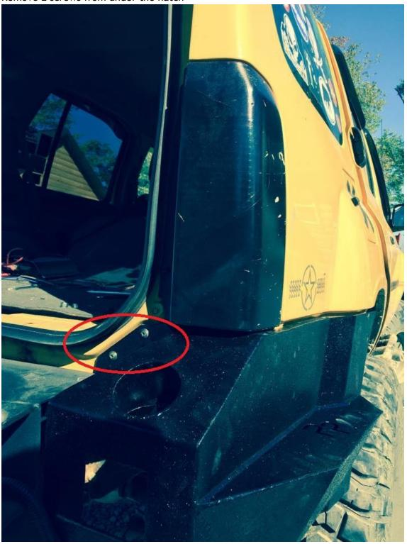
c. Remove lower support attached to pinch weld at bottom of truck
