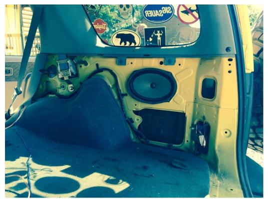
(3) Drill Holes on Pass. Side for Inner mounting plate
