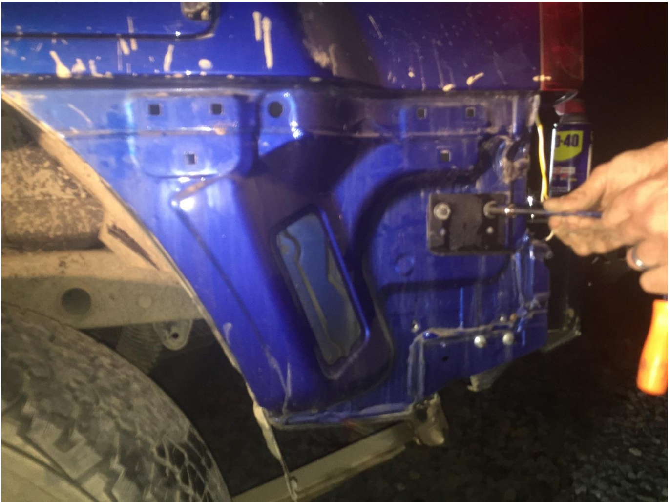
Figure 2c – P&P Engineering Corner Support Bracket on truck with only 2 main bracket holes
