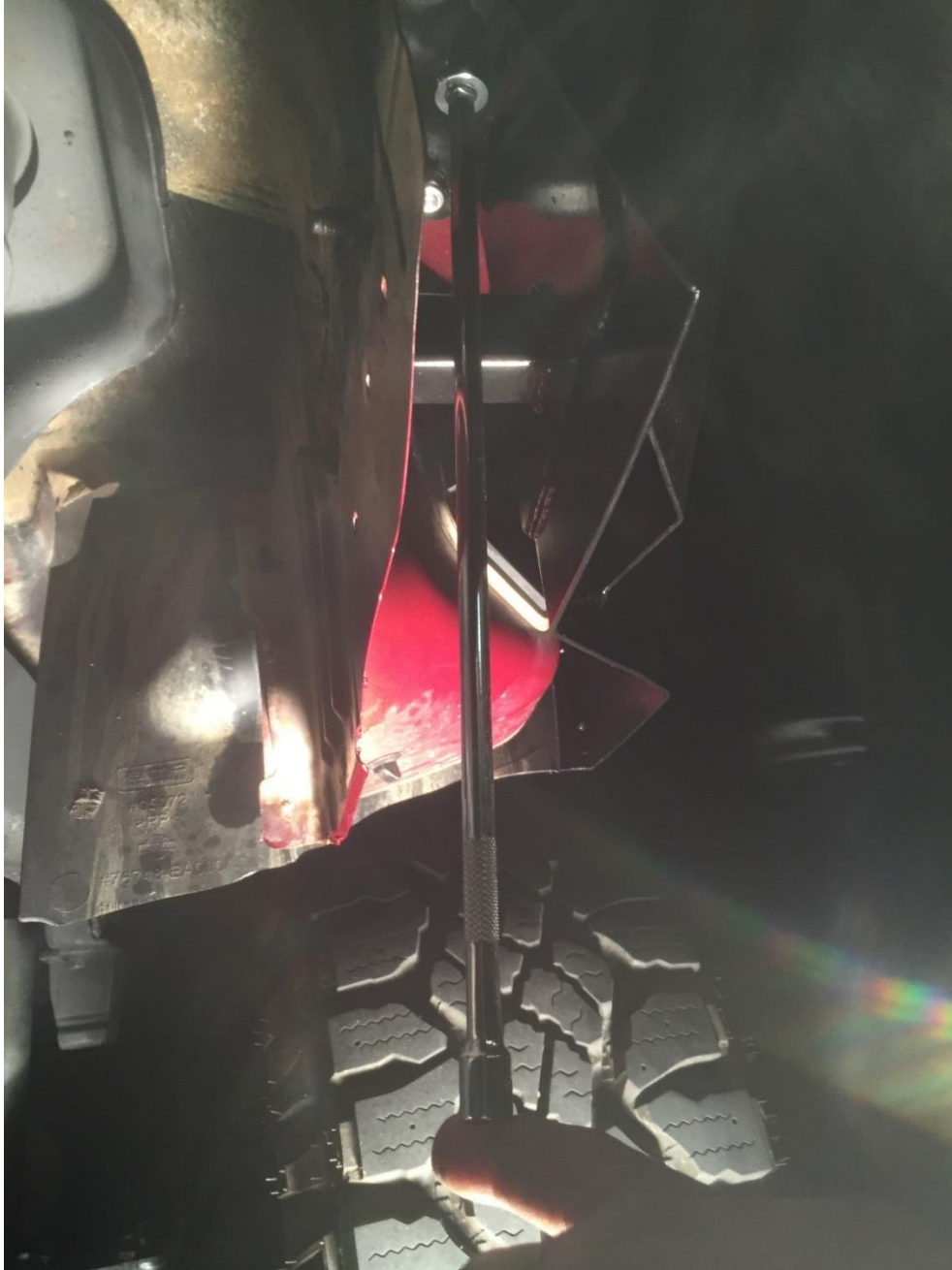
Figure 7 – A long extension is used to tighten nylock nuts on carriage bolts used in main support bracket.
