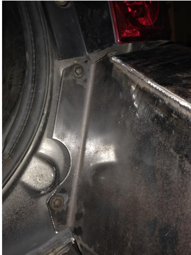
Figures 5a & 5b – Rear alignment flange with factory hardware
